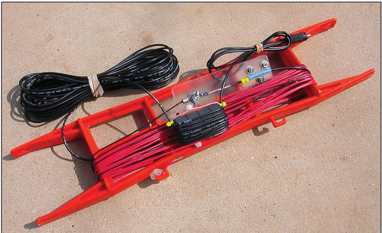
All wound up and ready to go, the trail-friendly version of Kurt N. Sterba's End-Fed Dipole Lite fits easily in a backpack and won't weigh you down on the trail. (Photos courtesy of KI6SN)
