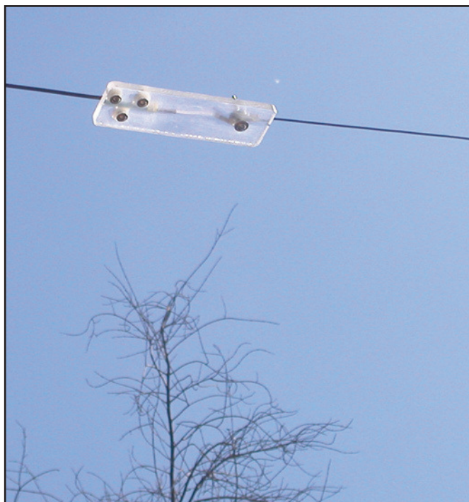
The Plexiglass center piece is the connection point for the RG-174U coax and No. 22 stranded hook-up wire in the trail-friendly End-Fed Dipole Lite.
