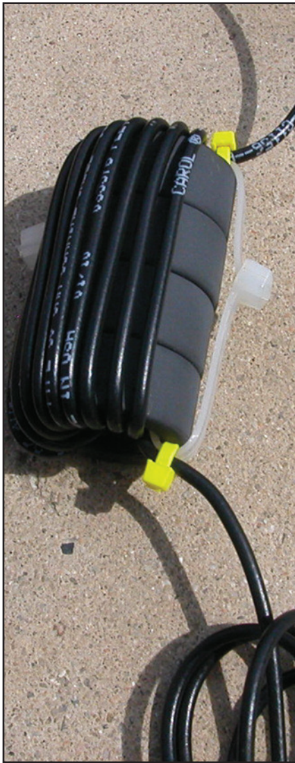
Stacked F114-61A toroids are one of the secret weapons of the trail-friendly End Fed Dipole Lite. Nylon wire ties hold the ferrite cores and coax in place.
